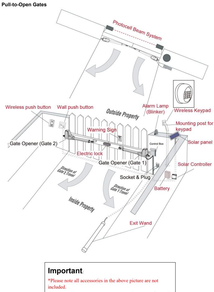
The second gate opener cable should be put into the PVC conduit (not provided) which is huvid underground. This protects the
