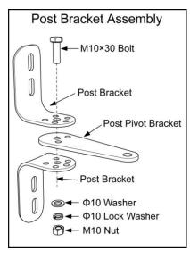
**1.** Insert the M10 x 30 bolt through the center hole of the post bracket and post pivot bracket as shown. Place a  $\emptyset$  10 washer,  $\emptyset$  10 lock washer and M10 nut on the bottom of the bolt and hand tighten.
