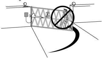
8. Pedestrians should never cross the pathway of a moving gate. The gate opener is not acceptable for use
