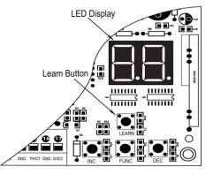
NOTE: Max. 8 remotes can be programmed for the opener. An External Receiver (optional) allows up to 250pcs remotes to be programmed for the opener. The external receiver is also compatible with other brand swing gate opener, sliding gate opener and garage door opener.
