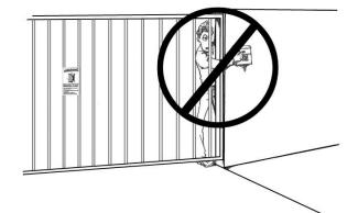
11. Controls intended to be used to reset an operator after 2 sequential activations of the entrapment protection device or devices must be located in the line of sight of the gate, or easily accessible controls shall have a security feature to prevent unauthorized use. Never allow anyone to hang on or ride the gate during the entire travel of the gate.
