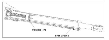
cold climates where temperatures reach 1°C (30°F) or less, spray silicone on the actuator every 4~6 weeks to prevent freeze up.
