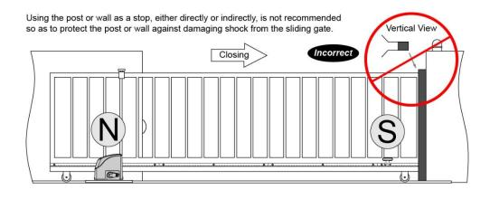
For the sake of safety, a positive stop must be mounted at both ends of ground track.
