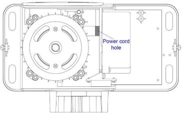
**2.** Prepare one or more conduits for the electrical cables before pouring concrete. Remember that cable conduits have to pass through the hole in the opener base.
